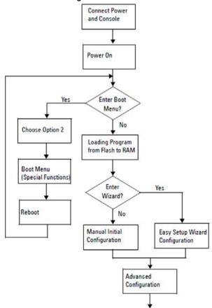
Figure 1-5. Installation and Configuration Flow Chart
